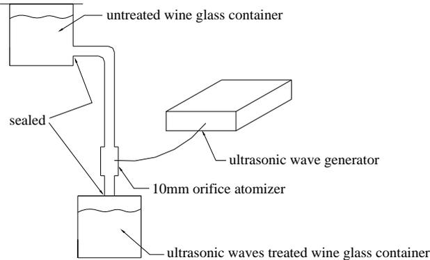
Figure. 1 Diagram of the ultrasonic waves set up
